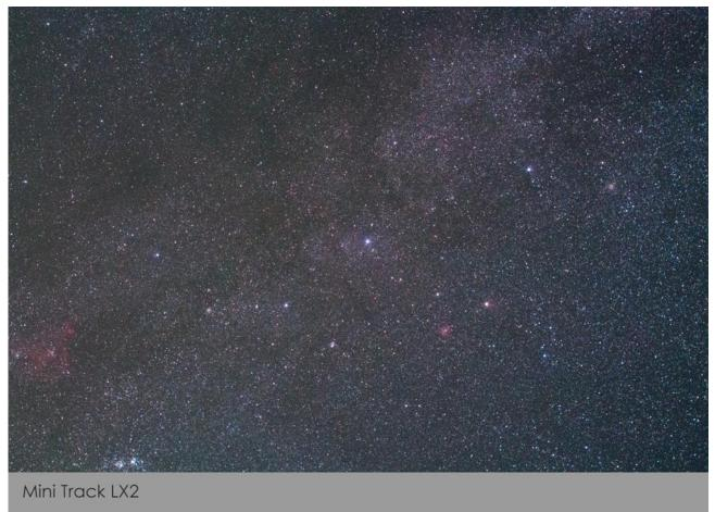
Test of the spring system, 13.10.2018, Austria Constellation Cassiopeia, single shot, no darks, no flats 50mm focal length @f/4, EOS 1100Da, ISO3200, Neodymium lens filter, 2min exposure, payload weight (body & lens) 0.8kg Camera in extreme position west of the tracker pointing at the zenith, spring set to position R
