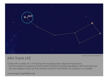
If the instrument pole is within this circle of 2.8 degrees diameter around the celestial pole, no trailing due to polar misalignment will occur. This coarse alignment precision of +/-1.4 degrees can easily be achieved with the sighting tube. If the sighting tube is carefully oriented toward Polaris, any trailing that remains is most likely due to other causes, like errors of the clock drive, slippage of the ball head, strong winds, an unstable surface or flexure of an overloaded tripod.
