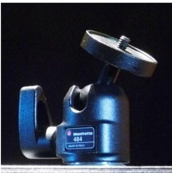
**Use a Heavy-duty Ball Head:** The ball head is the point most likely to show flexure. So, don't betray the high accuracy of your Astrotrac system by using a ball head too weak. The ball head has to support the full weight of your DSLR including its lens. When imaging with optics in the range of 200/300mm focal length, the total camera weight can amount to 3kg or more. Before selecting a ball head for your Astrotrac system carefully study its specs, especially the maximum weight supported.
