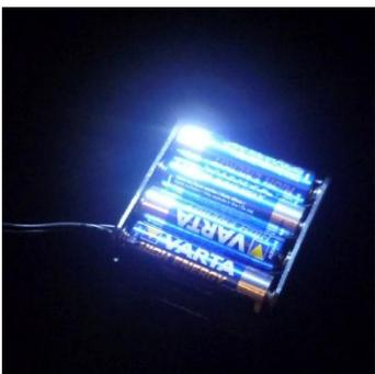
**Use the Battery Holder:** With the battery pack loaded with a set of 8 alkaline AA batteries the Astrotrac runs for about 8 hours. The battery holder gives you freedom of external power sources, a fact that can't be valued enough when it comes to mobility. We recommend keeping the battery holder inside a small camera bag, available in any camera store. This keeps the batteries away from the often inevitable dew.
