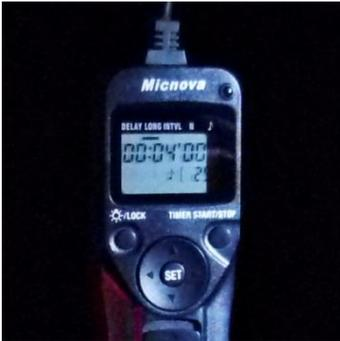
**Use a Timer:** The Astrotrac system runs fully automatically for hours. To automate the entire imaging process an additional camera timer is needed. With a device like this it is possible to program a series of exposures. After that, the push of a button starts an automated imaging sequence. This leaves you plenty of time to enjoy the beauty of the night sky.
