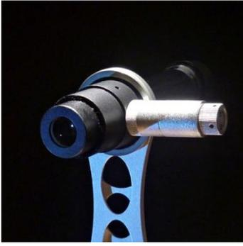
**Focus the Polar Scope:** To achieve high accuracy polar alignment it is necessary to work with a well-focused polar scope - meaning that objects at infinity (e.g. Polaris) and the reticle marks have to look sharp at the same time. Adjust your polar scope until this is the case. Otherwise, tiny movements of your head will cause the alignment stars to shift against the reticle marks and your polar alignment will not be precise.
