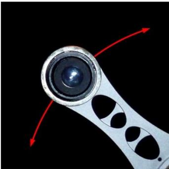
**Collimate the Polar Scope Arm:** The polar scope must always stay parallel with the Astrotrac's axis. Again, aim the polar scope at a terrestrial target. This time, rotate the polar scope arm and notice the target's movements. To eliminate the target's movements, small pieces of duct tape can be applied between the polar scope and the polar scope arm. Once you've found the right positions for the tape strips, stick them permanently to the polar scope arm.
