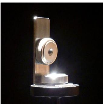
**Restore Freedom of Camera Orientation:** Using the Astrotrac with a ball head is sufficient to aim the camera at any point in the sky. However, for the area between the celestial pole and the zenith the camera does not have full freedom of orientation. A simple 90° angle bracket between the camera and the ball head solves this problem and restores the full range of movement in this section of the sky. Since such brackets are not available as standard equipment, we customised one ourselves.
