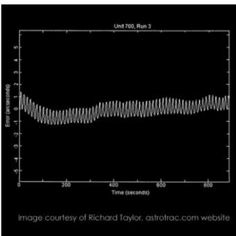
**Trust the High Precision Tracking:** The manufacturer claims a tracking precision of 5 arcseconds peak-to-peak within 5 minutes. We field-tested our Astrotrac unit for tracking precision and found exactly the same value. So if there are trailed stars on your images the reason most likely is not bad tracking precision. Trailed stars hint that either your polar alignment was off or a part of your mounting hardware (e.g. tripod, ball head,...) showed flexure.
