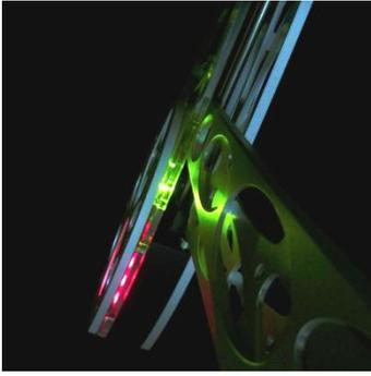
**Avoid the Astrotrac Light Trap:** For those imaging with a DSLR there is a nasty trap built into the Astrotrac system. It goes by the name of green flashing status light. Some camera positions allow this green light to enter the camera body through the viewfinder, which later shows on the images as a faint green glow. In any case it is very wise to cover the camera body's viewfinder during the actual exposure series.
