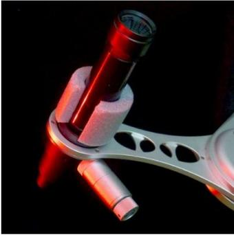
**Secure the Polar Scope:** During operation, the polar scope is held in place by three tiny magnets on the underside of the Astrotrac's polar scope arm. Since the polar scope arm and the camera body are in close vicinity to one another, it is easy to bump into the polar scope, especially in the dark. To prevent it from falling down (and losing its collimation, to name the least) a short piece of 3/4 inch tubular pipe insulation can be used. Simply snap it on to the polar scope.
